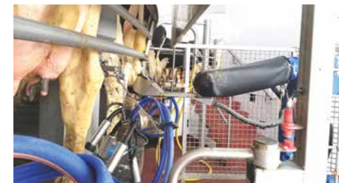
This robot is used to dip udders before cows leave the carousel at Heiman's Holsteins.
